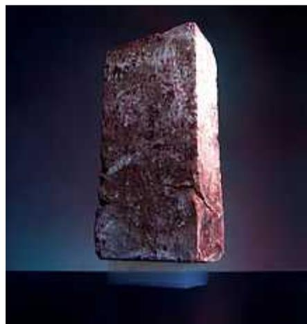
*A 2.5 kg brick is supported by a piece of aerogel with a mass of 2 g.*
